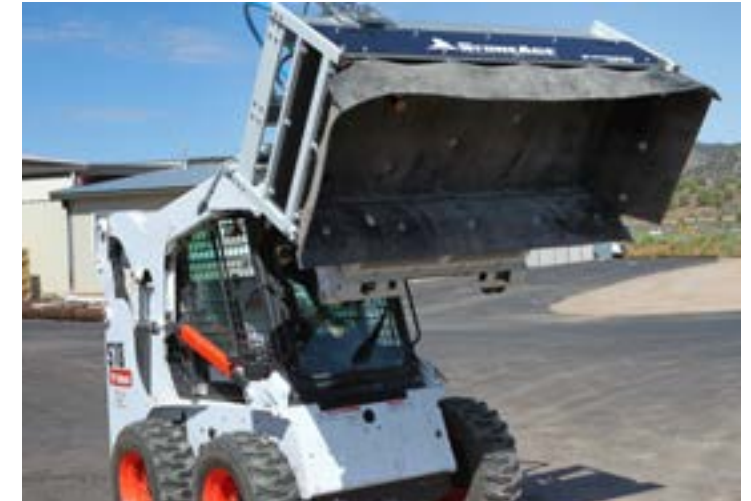
Rubber lined shroud reduces noise and contains debris
