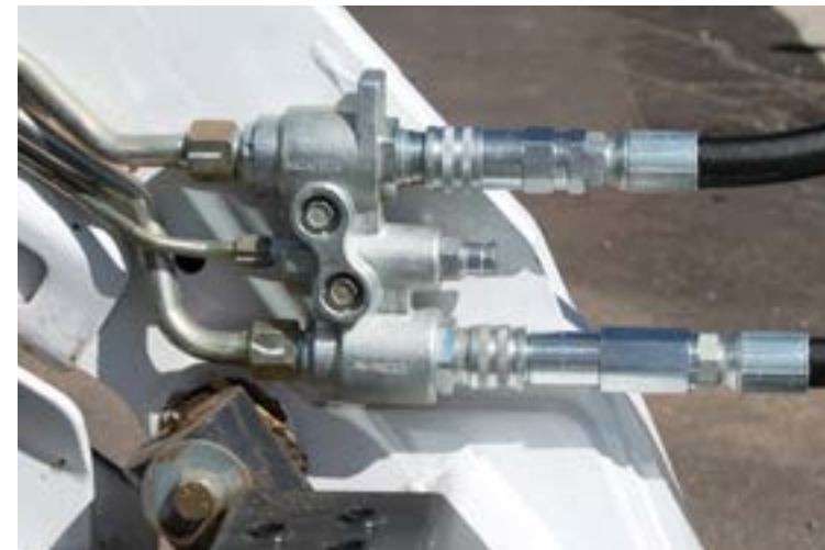
Supplied quick connectors attach to most standard flow skid steers
