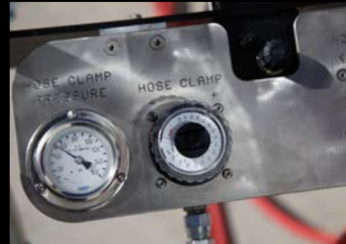
Pneumatic controls remotely adjust hose clamp pressure, hose feed speed and hose feed direction (forward/reverse)
